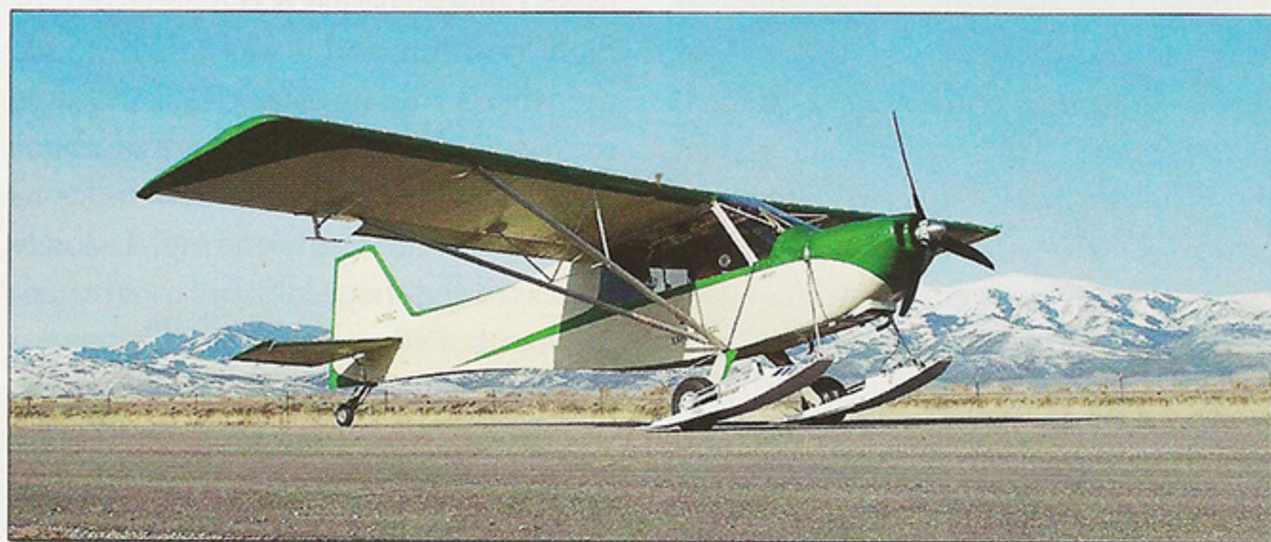
One of the rare times the plane was on asphalt; the skis are well clear, and wheeled ops are normal. The author misses his big fat 26-inch Airstreaks, though.
