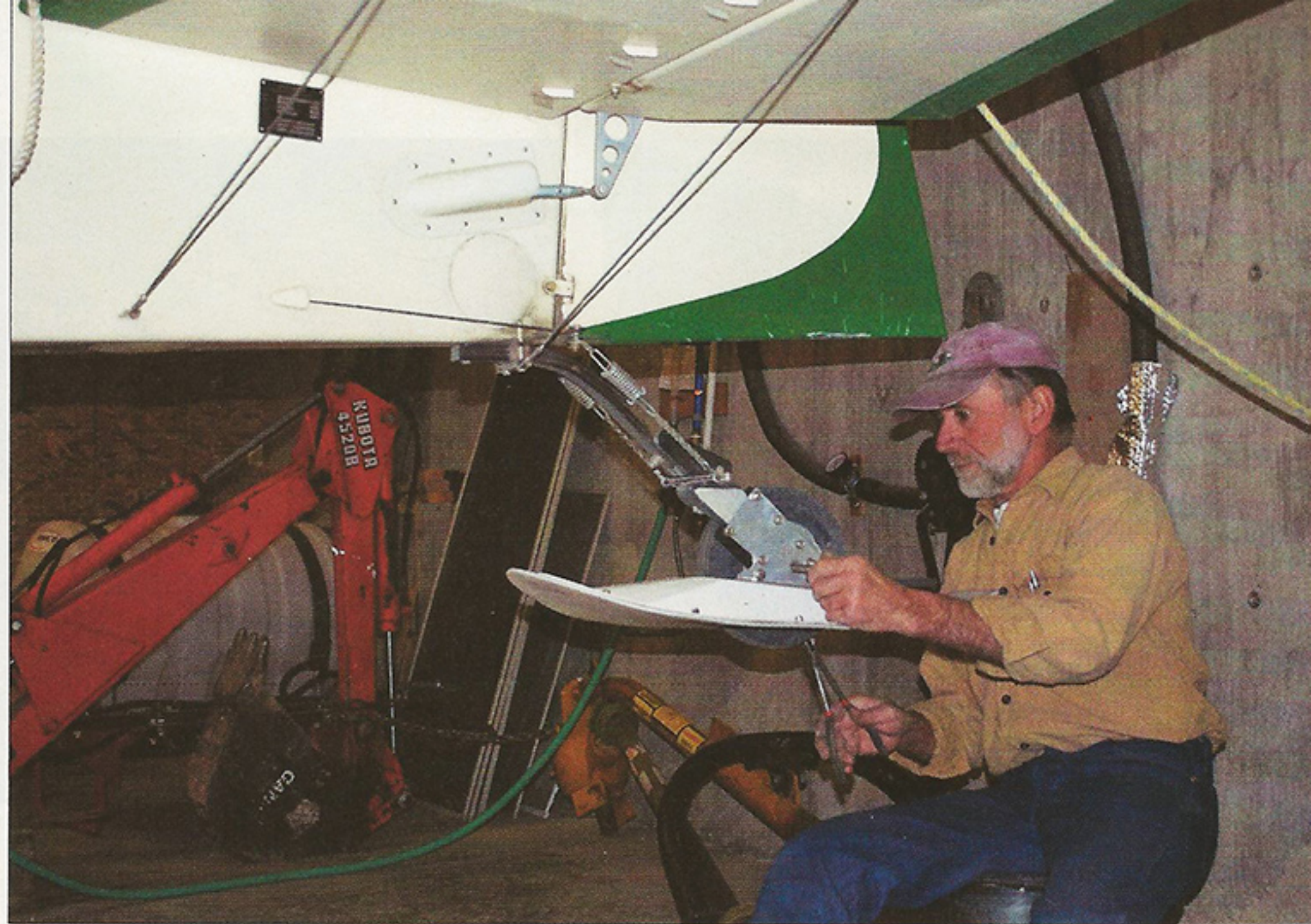
Simko reinstalls the tailwheel ski.
