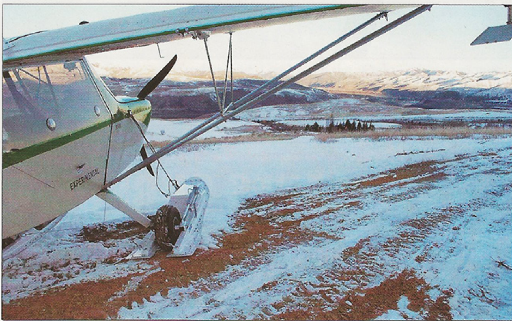
A good example of why Simko wanted wheel/skis, and not simple skis. He routinely has to deal with pavement, gravel and deep snow—all in the same flight.
