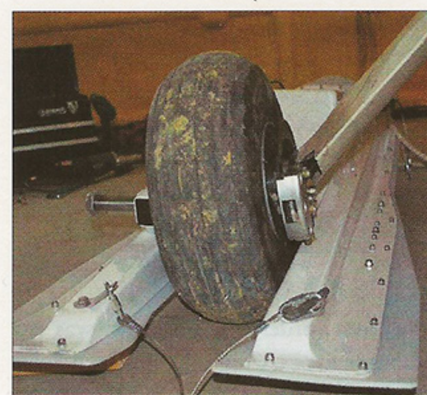
This photo shows that the brake caliper would have interfered with the ski before it was moved.
