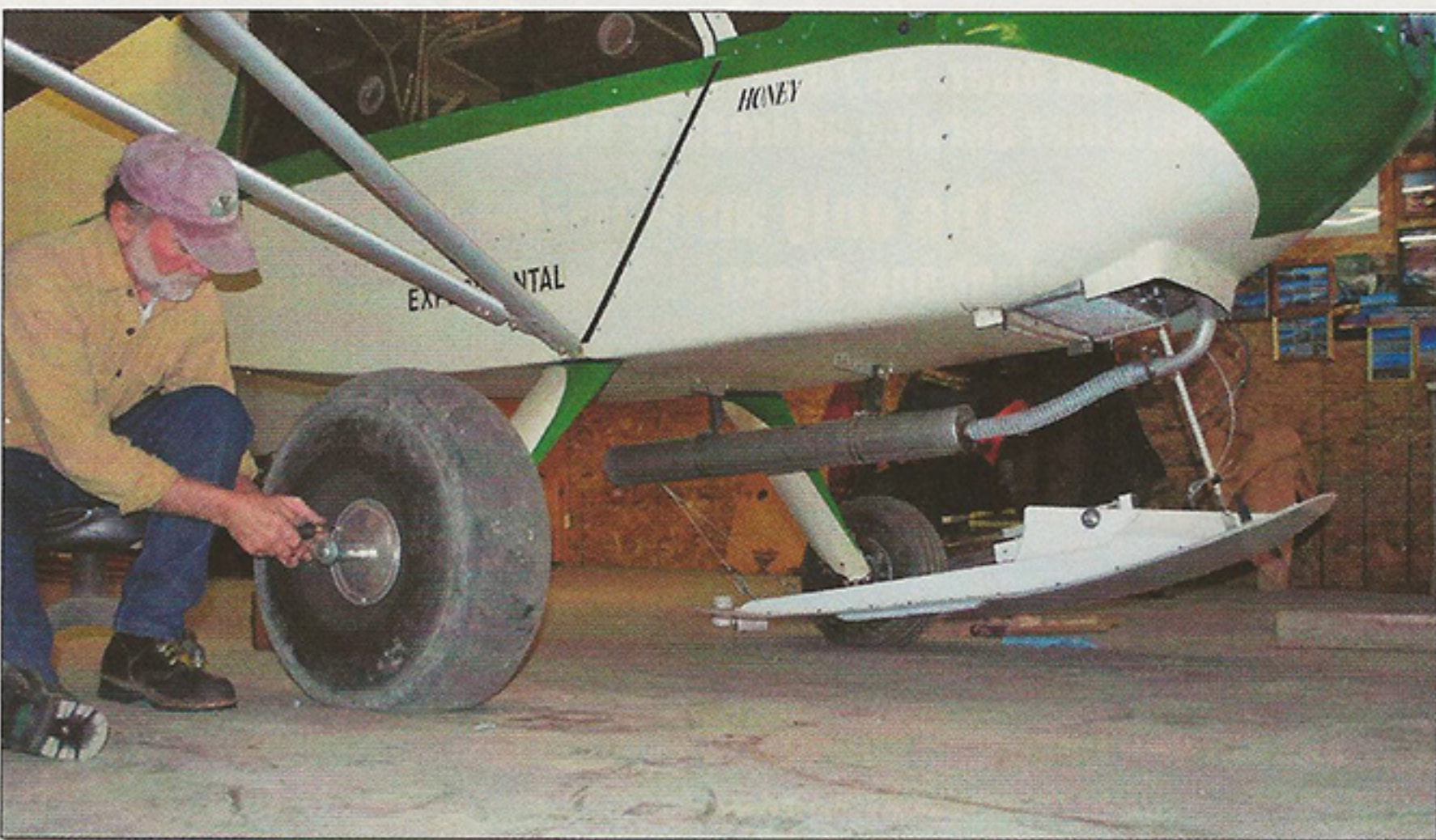
Off come the 26-pound Airstreaks in favor of the lighter 6.00 tires.
