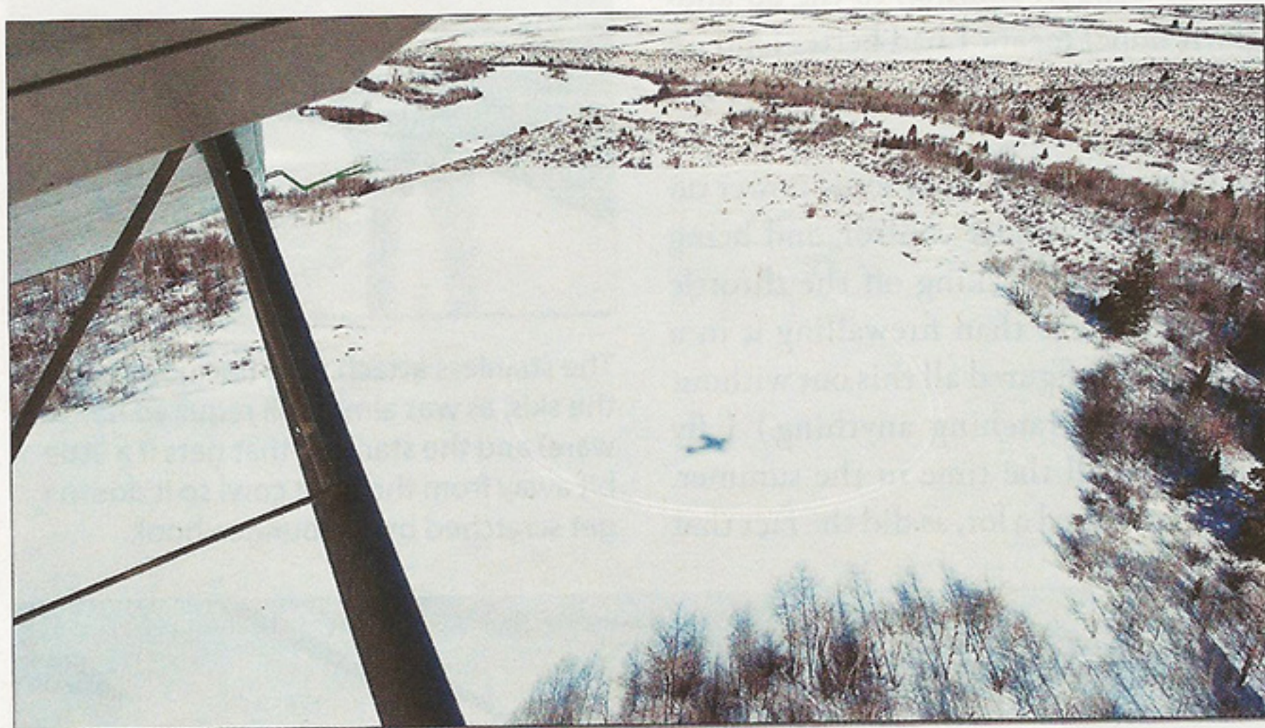
The tracks show the landing and, more important, the turnaround, which is especially tricky on the mountain slopes. Once the turn is started and you're headed back downhill, you are committed—no brakes!
