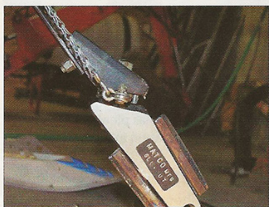
Two views that show more of the tail ski attach bracket.
